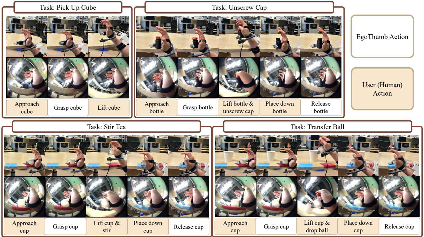
Fig. 3: Execution Sequences for the Four Evaluation Tasks. Policy rollouts demonstrating collaborative human-robot manipulation across four tasks: Pick Up Cube , Unscrew Cap , Stir Tea , Transfer Ball . For each task, the top row displays the user’s first-person view of the interaction, while the bottom row shows the corresponding egocentric palm-facing camera view used by the policy. The timelines below outline the coordinated sequence of autonomous EgoThumb actions and human motions.
